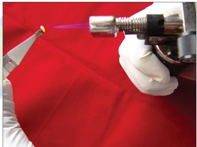
Figure 4: Burning old bonding material
