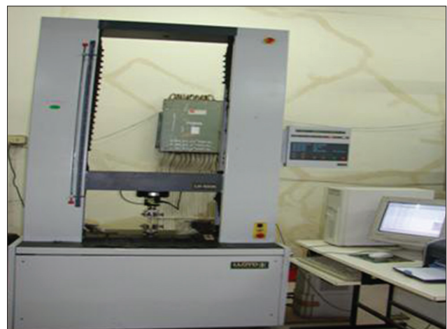
Figure 2: Lloyd universal testing machine
