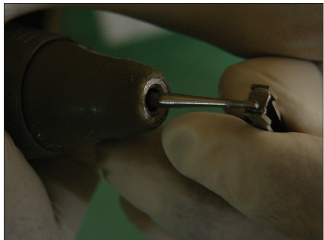
Figure 6: Adhesive grinding using tungsten carbide bur
